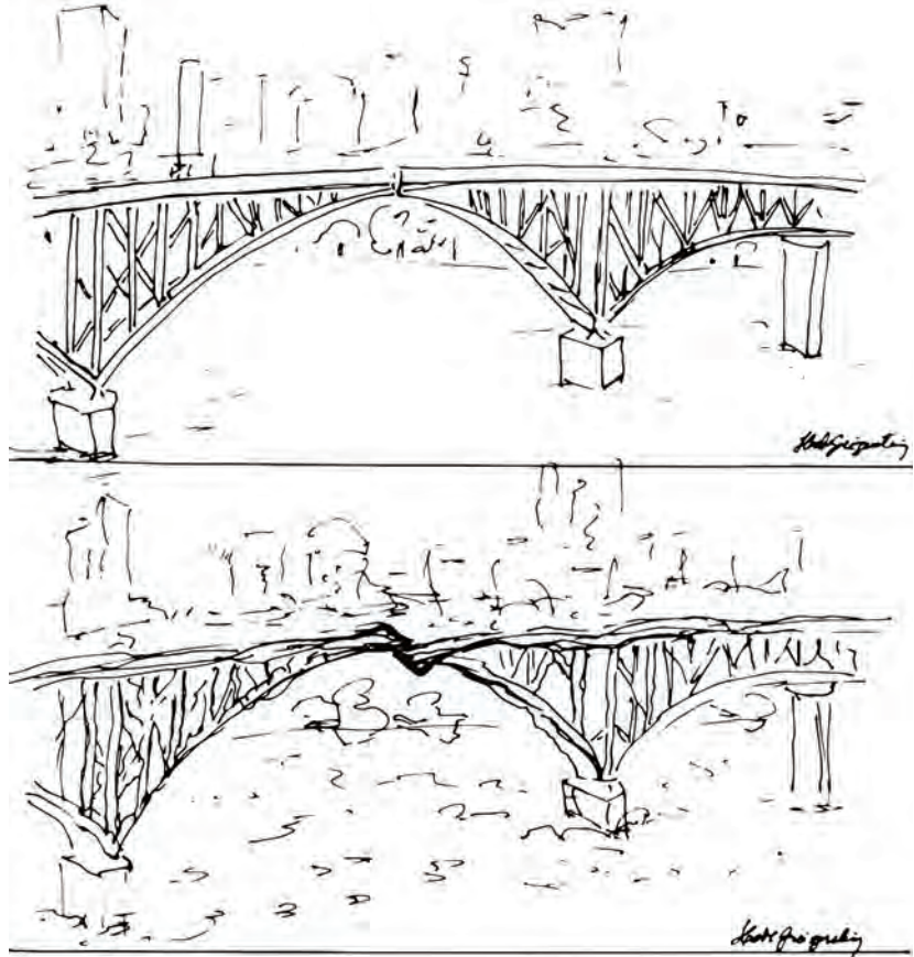
The Ross Island Bridge, top, is Portland’s weakest. It is not expected to survive earthquake without major damage, bottom. Illustrations by Hebe Greizerstein
