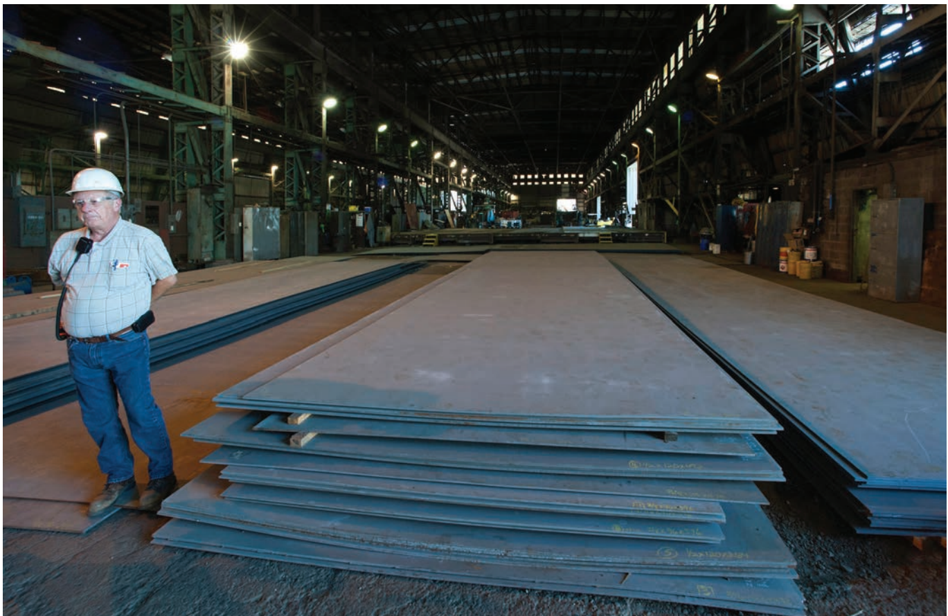
Tony Hoppe stands by a barge “Do It Yourself Kit”-the sheets of steel from which the 3,000-ton barge is made.
