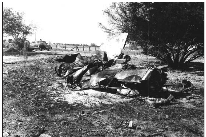
The rest of the wreckage. Everything landed on government property. The wing center section was recovered out of the wreckage, was tested and failed again.
