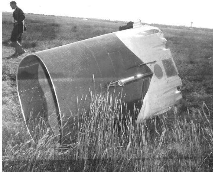
The intake (first six feet) of the aircraft blew off when the aircraft engine exploded.
