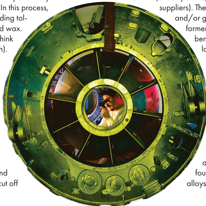
This is the 76-inch diameter airplane component that Precision Castparts claims is the world's largest cast metal object."
